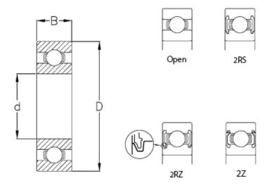
B = 10 Ball grade = 5 C (KN) = 4.94 C0 = 3.15 d = 17 D = 35 Max rpm. = 13000 Type = 6003
